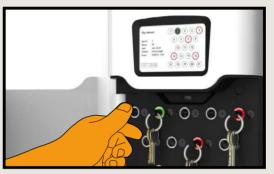
All keys and keysets are individually locked by the Traka21 unit. Green LEDs indicate those keys to which this user has access. The user cannot remove keys highlighted by the Red LEDs which continue to remain locked in place.
