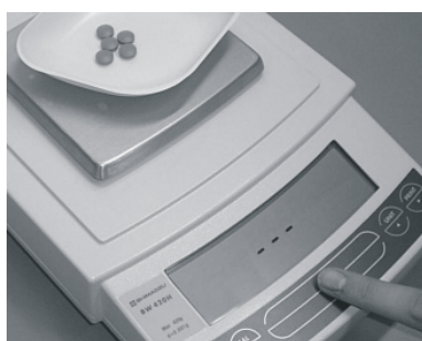
Place the sample on the pan
